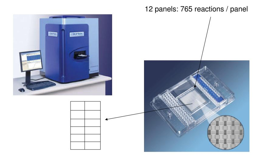
$2.5 \,\mu$ l DNA (5ng/ $\mu$ l or 40ng/ $\mu$ l) was added to a PCR mix and loaded onto individual panels of the digital array. qPCR was performed and individual reactions that contained a D816V molecule are detected.
